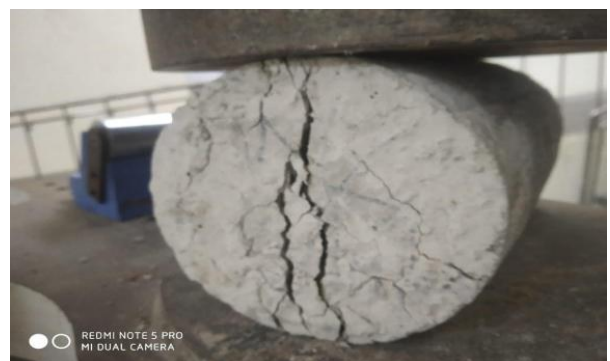
Fig -4 Formation of Various Crack on the Cylinder
