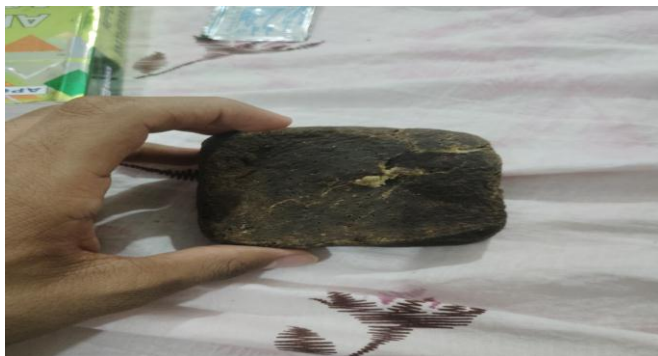
Fig -1: TRIAL WITH EXCESS HARDENER
