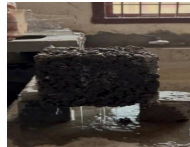
Fig -10: Infiltration testing
