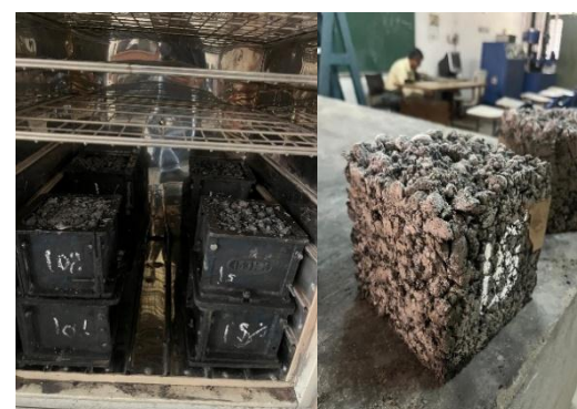
Fig. -8 Samples in oven for curing and demoulded sample
