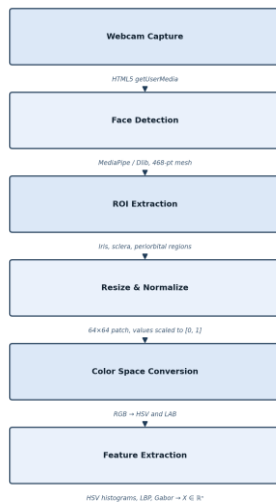
Fig. 2. Data collection and preprocessing pipeline: webcam capture through feature extraction.
