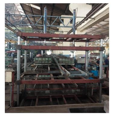
**Hydraulic System:** At the heart of the hydraulic mold box lifter is a hydraulic system. This system consists of a hydraulic pump, hydraulic fluid, hydraulic cylinders, control valves, and piping. The pump pressurizes the hydraulic fluid, which is then controlled and directed by the valves to the cylinders.
