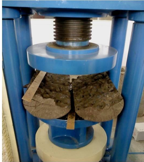
Figure 4.1 Splitting of cylinder
