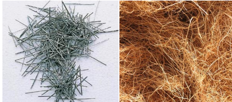
Figure 3.1 Steel fibre and coconut fibre
