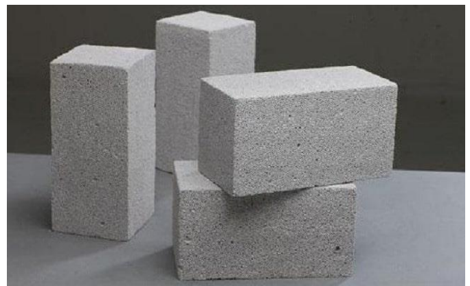
Figure-1: Light Weight Concrete.
