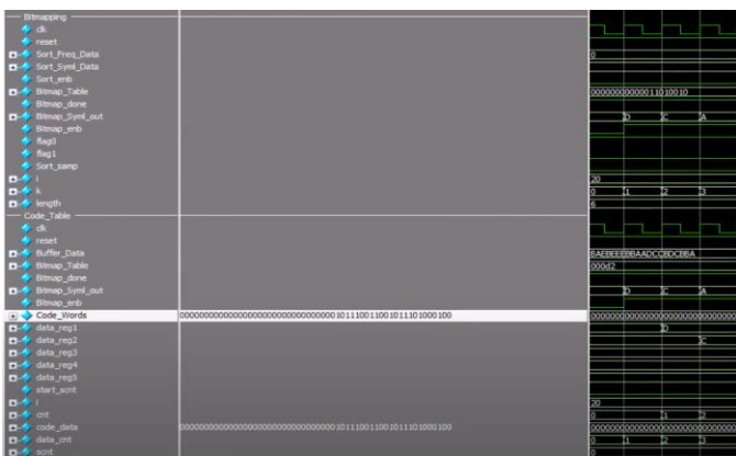
Fig8: simulation waveform of code table module
