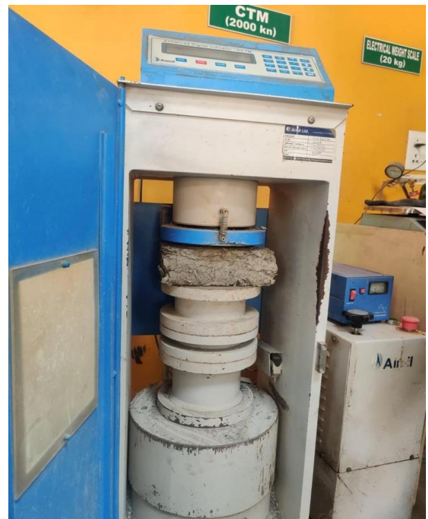
Fig -3: Compressive strength test on plastic bricks
