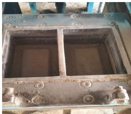
Fig -1: Brick Molds used for casting of plastic bricks.
