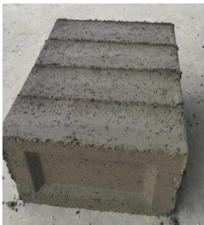
Fig -2: Manufacturing of bricks with plastic waste.
