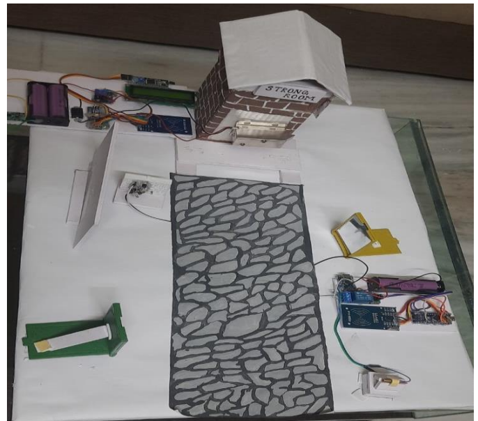
Fig -3: Laser Beam Alarm with an Automatic Door Lock System
