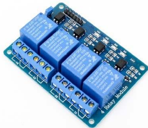
Fig: Relay board
