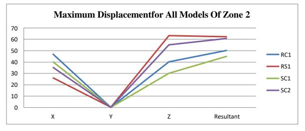
Fig. 5.1.3 Comparison of Maximum Displacement for all models of zone 2
