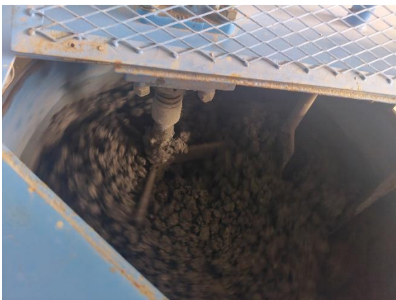
Fig - 1 Casting of Concrete in mixer
