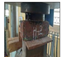
Fig -5: HDPE and PP Brick sample for testing
