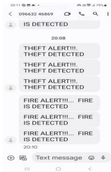
Figure[7]: Offline Alert Received on mobile phone through SMS
