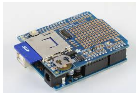
Fig -4: Arduino data logger shield physical figure.
