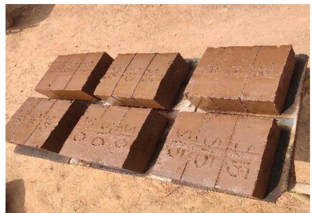
Fig -3: Wire cut bricks
