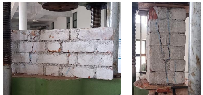
Fig -6: Failure of masonry specimens
