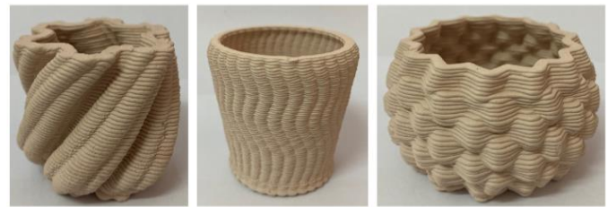
Figure 8: Printed model products with complex patterns
