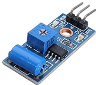
Fig -5: Vibration sensor
