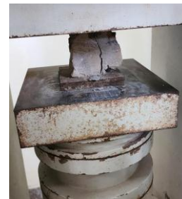
Fig -31: Onsite core samples were tested for compression
