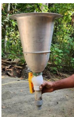
Fig -11: Concrete extruder fabricated with available resources
