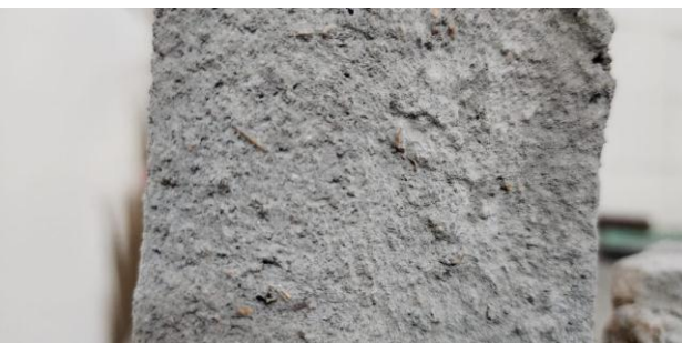
Fig -43: Enlarged section of Trial mix-02 sample: No cold joint, powdery surface texture.
