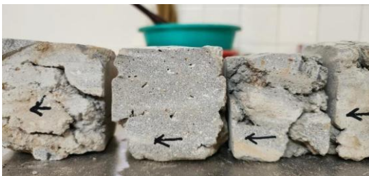
Fig -28: Core Samples taken. Print direction and top direction marked
