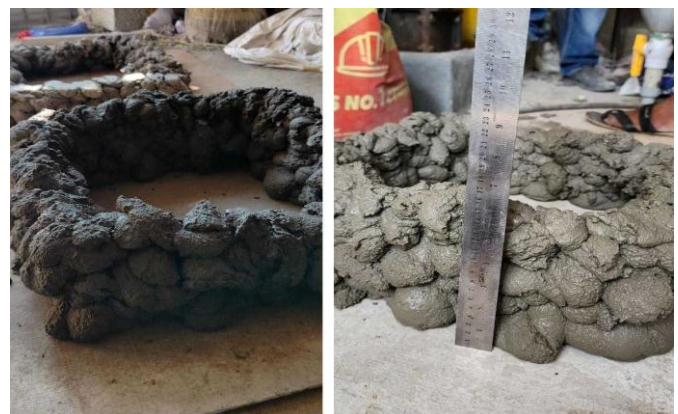
Fig -40: Left - Extrusion completed & Right - Improved Buildability with respect to Trialmix-01
