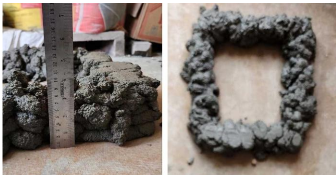
Fig -22: Left – Check for buildability, Right - Hand printed sample
