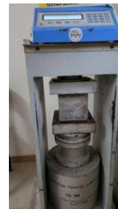
Fig -23: Compression test in progress
