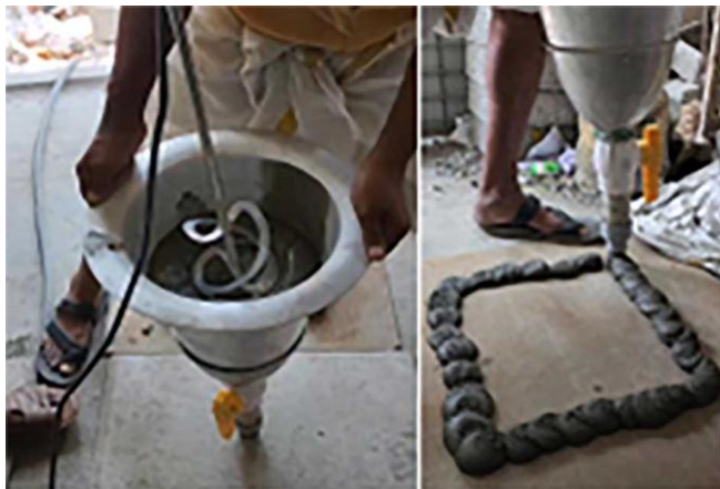
Fig -21: Extrusion by hand printer starts
