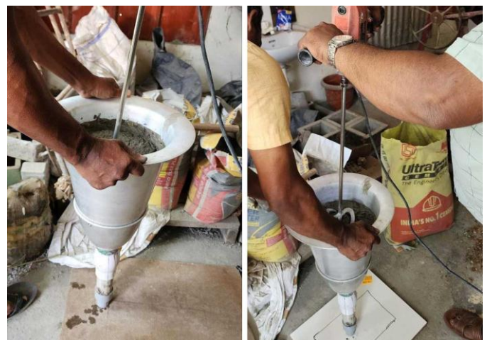
Fig -20: Left - Material mixed in extruder, Right - Extrusion test & check admixture dosage
