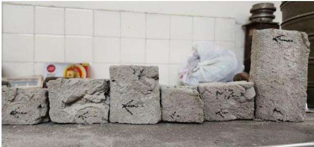
Fig -41: Core samples taken. Print direction and top direction marked.
