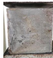
Fig -24: Cube crushed at 7 day & Cracking patterns studied
