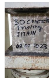
Fig -25: Cube crushed at 28day & Cracking pattern studied
