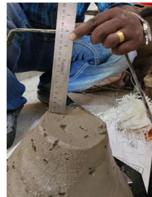
Fig -19: Measurement of Slump (Slump value observed =140mm)
