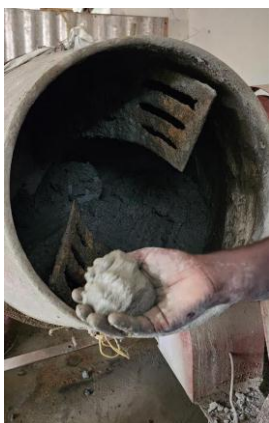
Fig -18: Trial Mix-01: Materials Mixed & consistency checked
