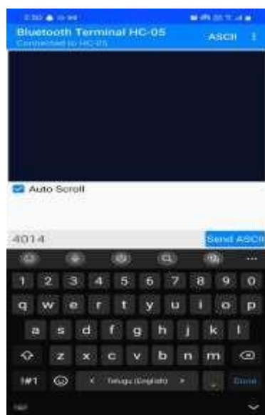
Fig -9: Bluetooth terminal HC-05
