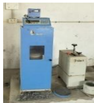
Fig 4: Aggregate crushing machine
