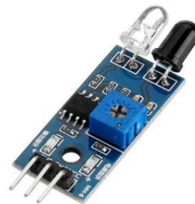
Fig-9: Infrared Sensor
