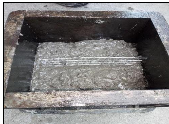
Fig -2: Wire mesh arrangement 2
