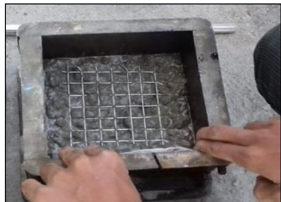
Fig -1: Wire mesh arrangement 1
