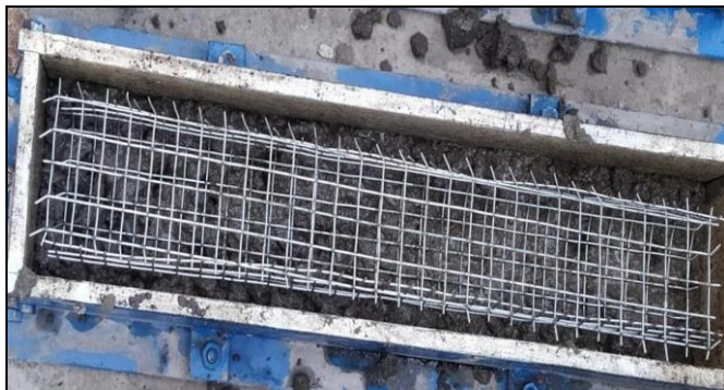
Fig -4: Wire mesh arrangement 4
