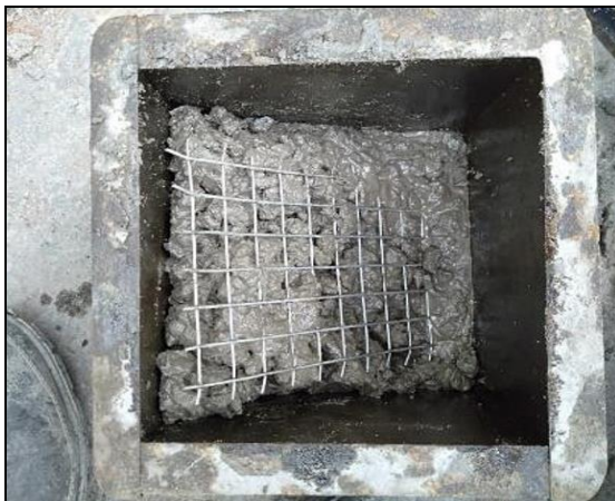
Fig -3: Wire mesh arrangement 3
