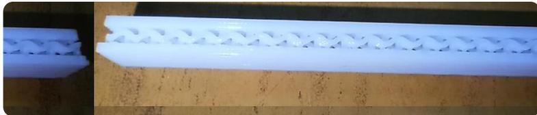
Figure 8 shows Gyroid Infill Pattern
