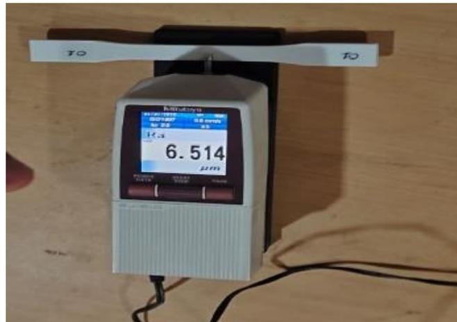
Figure 16 Surface Roughness Tester
