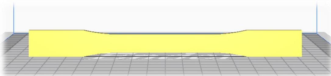
**Figure 4** demonstration of on-edge orientation
