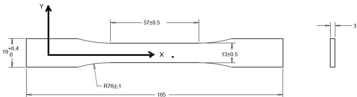
Figure 15 Demonstration of X and Y axis of FDM Specimens for Surface Roughness
