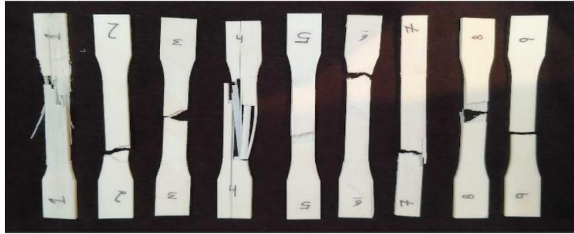
Figure 14 Tensile Tested FDM Specimens
