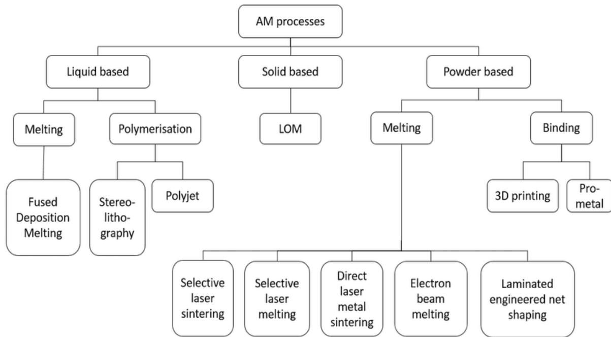
**Figure 1** Detailed classification of additive manufacturing
