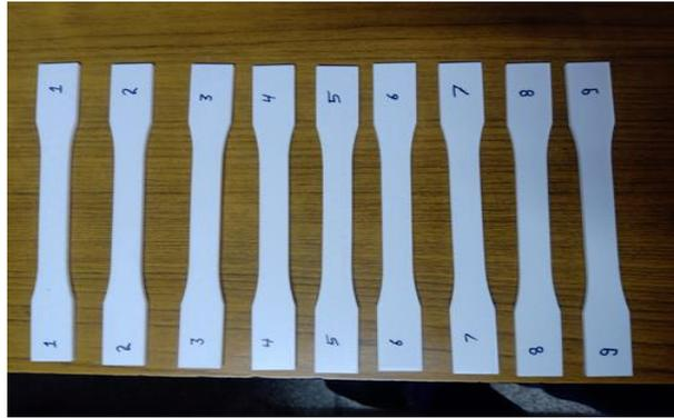
Figure 11 FDM fabricated specimens
