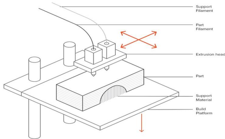
**Figure 2** Schematic of a typical FDM printer
