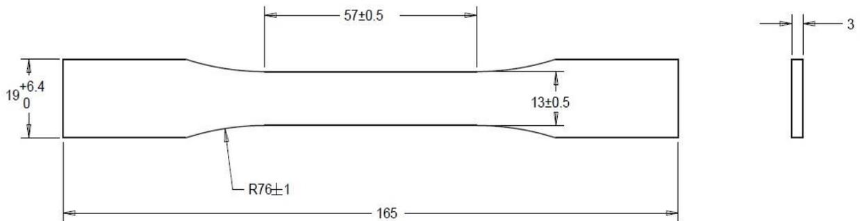
Figure 10 Specification of the specimen
