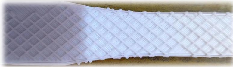
Figure 7 shows Cubic Infill Pattern
