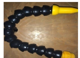
Fig -12: Coolant Pipe
