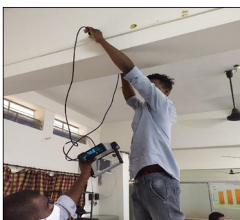
Fig.2 UPV test on RC beam
