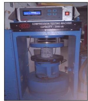
Fig.7 Concrete core compression test
