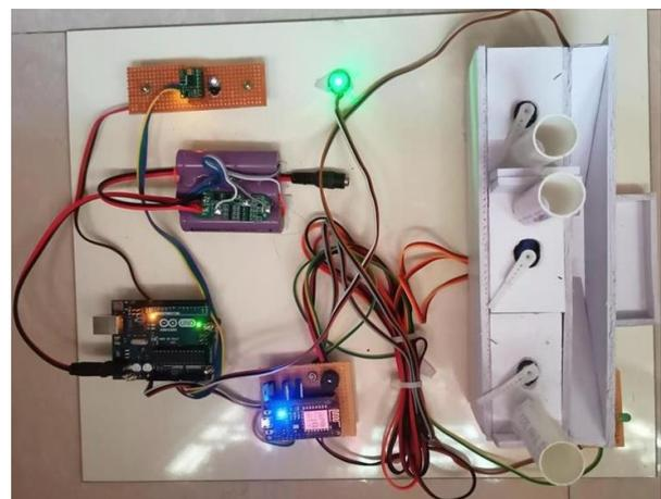
Upon rotation, the servo motor expels the designated tablet through the inclined pathway, directing it smoothly into the tray without spillage. The dispensation process is indicated by LED and buzzer alerts, providing visual and auditory confirmation of successful medication delivery. The presence of the dispensed pills in the tray is continuously monitored using an IR sensor, ensuring accurate tracking and management of medication intake.
