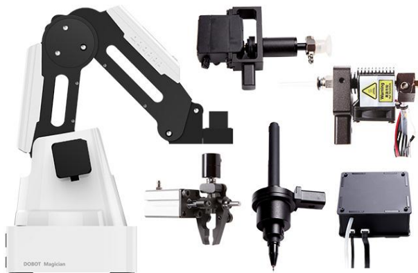
Figure 6. Different end-effectors of a robotic arm [31]
