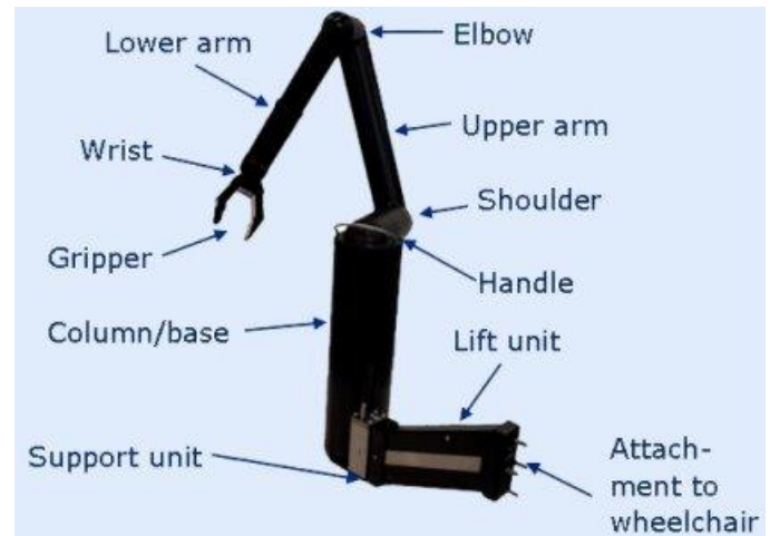
Figure 1. A robotic arm with labels [1]
