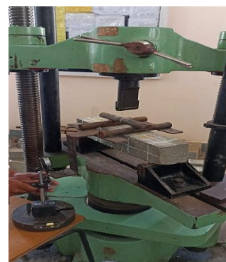
Fig No. a) Flexural strength test
