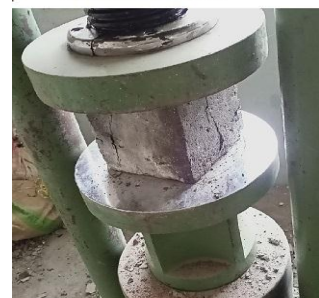
Fig No. c) Comprehensive strength test
