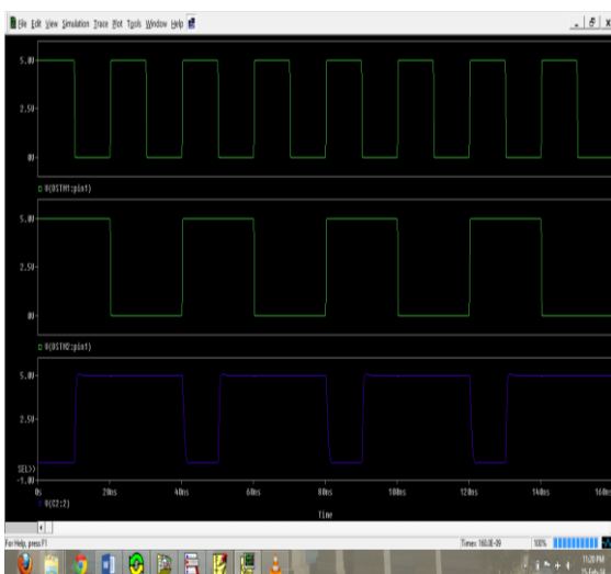
Fig4: Simulated input and output wave form of CMOS NAND gate (a) Input voltage V_A = V_{DSTM1} & V_B = V_{DSTM2} (b) Output voltage = V(C2:2)
