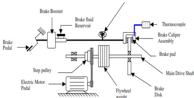
Figure 2: Schematic representation of the Brake pad test rig [4]
