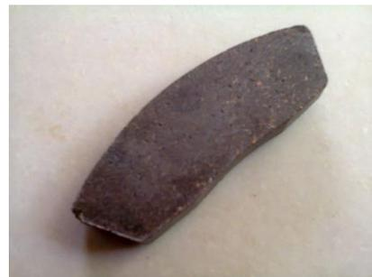
Figure 1 Sample brake pad after final finishing
